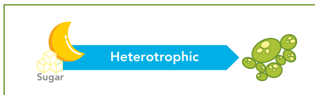
Figure 6: Heterotrophic microalgae are grown in large fermenter tanks using sugar or starch, similar to corn ethanol fermentation.
