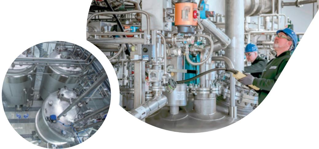
**kd-pür® Enhanced Silver Technology** is a further development of the kd-pür® technology, where ultra-high concentrations of EPA, DHA, DPA and other specific Omega-3 components can be achieved. This technology uses the supercritical carbon dioxide method and also includes a silverbased extraction process.
